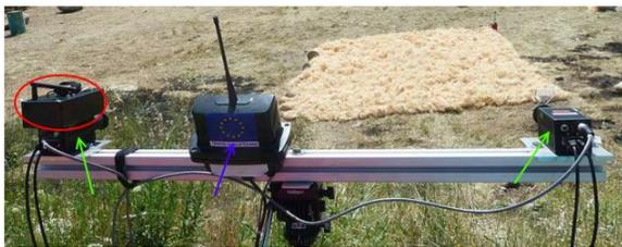
Fig. 1. 3D infrared-visible stereo system
