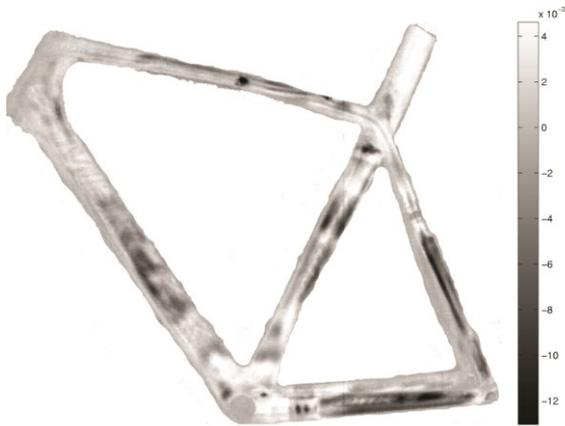
Fig. 5: Result of active thermography measurement after Principle Component post-processing.
