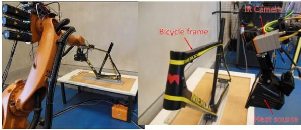
Fig. 1. Robotic thermal inspection on a CFRP bicycle frame.
