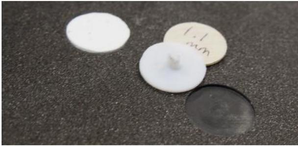
Fig. 3. Picture of the reference standard from the backside with flat bottom holes and the corresponding plug.
