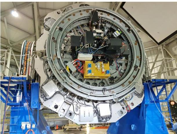
Fig. 5. IGRINS on the 4.3m Discovery Channel Telescope at Lowell Observatory. The cryostat is the gold box on the left. The three protruding blue boxes contain the Teledyne JADE2 USB interface cards. The CTI cold head and vacuum pump fitting are at the center of the side facing the reader. To the right is the electronics rack which holds the three detector computers and other auxiliary hardware. The black metal box
