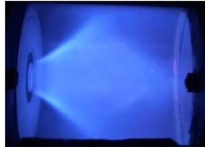
Figure 5. RGB image of flame luminosity showing a swirl stabilized flame inside the combustor.
