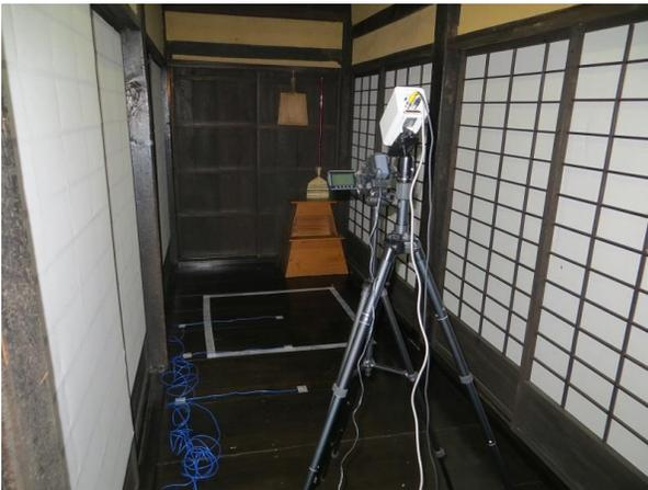
Fig. 2. Shooting scene with infrared camera.
