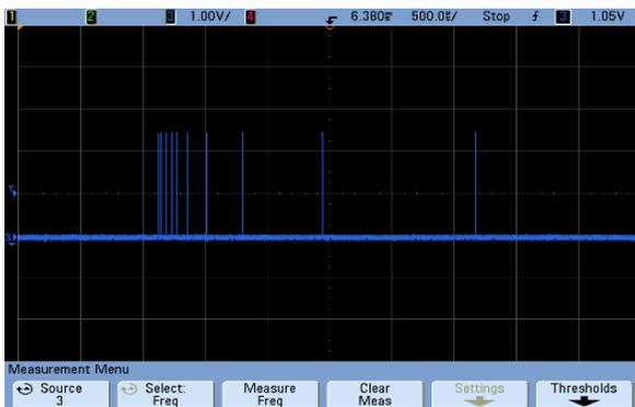
Fig.13(a) The waveform of the RST\_ACTIVE signal fed back by the DMD
