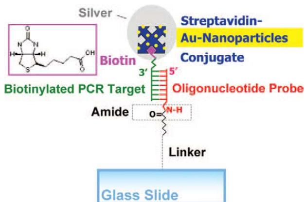
Fig. 2. Schematic illustration (not to scale) of the probe-target DNA duplex structure that enabled detection by IRCI.
