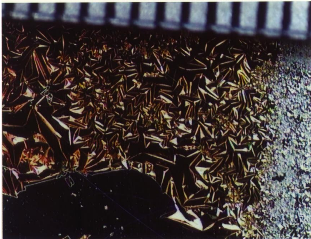
fig 6 : mirror macrophoto showing waves for the two thicker deposits 450 (right) and 550 (left) . on the upper part scale is shown : two black lines are separated by 1 mm .
