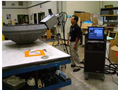
Fig. 4. Photograph of OV-105 Nose Cap inspection being performed by NASA LaRC personnel at Lockheed Martin Missile and Fire Control facilities in Dallas, TX.
