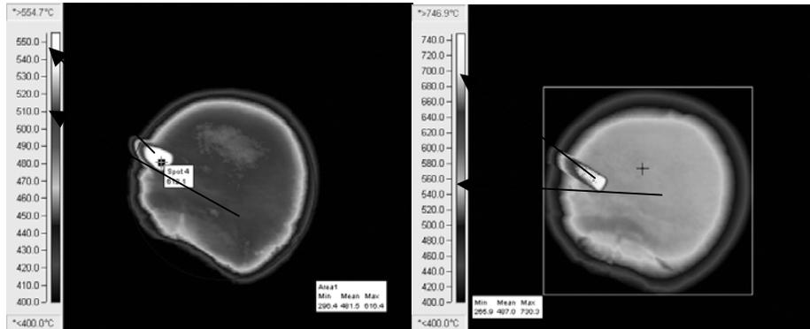
**Fig.4.** Ignition moment of di-methyl-ether inside the furnace.
