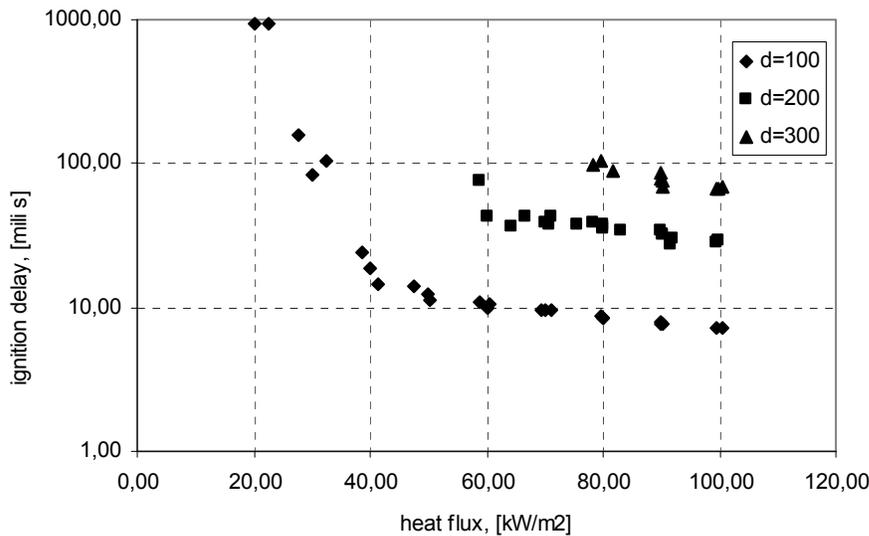
**Fig.2.** Ignition delay of the wood refuse versus DME.
