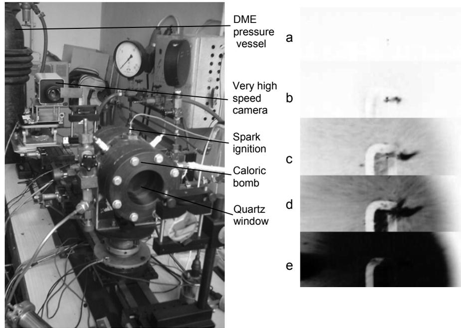
**Fig.1.** Experimental installation to test the ignition parameters for the mixture wood refuse and di-methyl-ether and a series of obtained images at 16500 frames/second.
