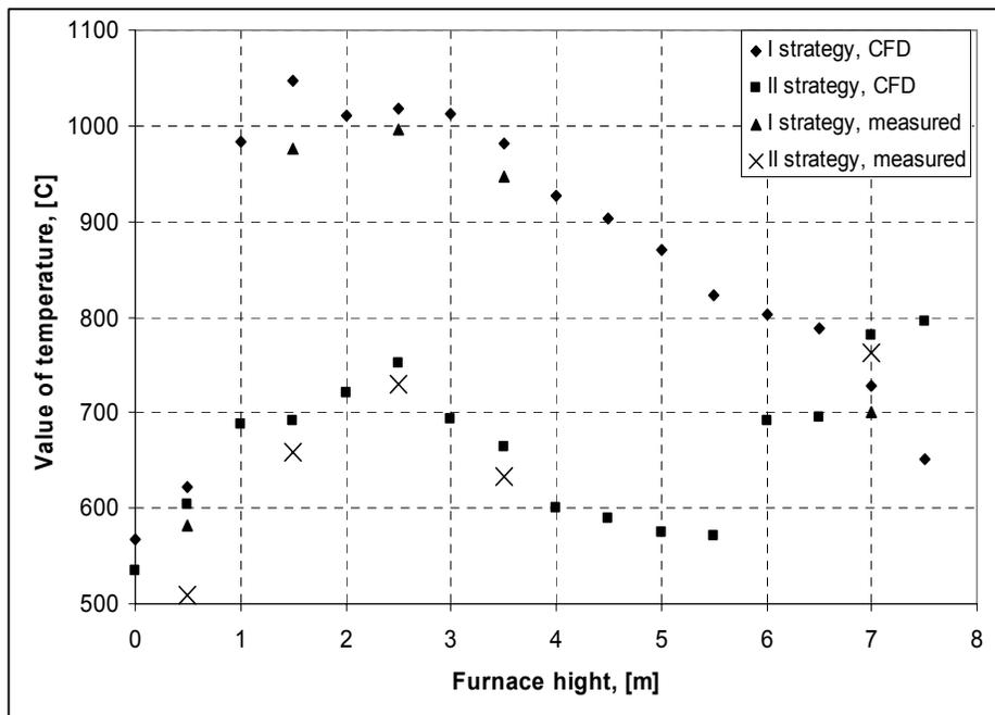
Fig.7. Measured and CFD predicted values of the temperature along the furnace height.
