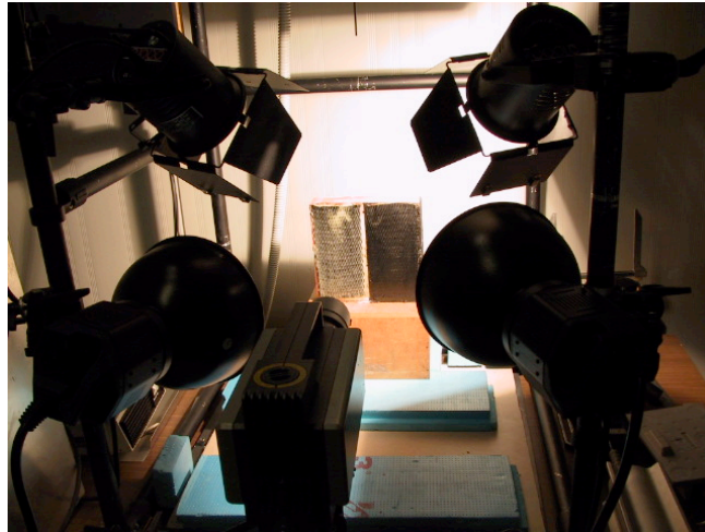
Fig. 6. Dynamic thermography set up during the heating of the sample
