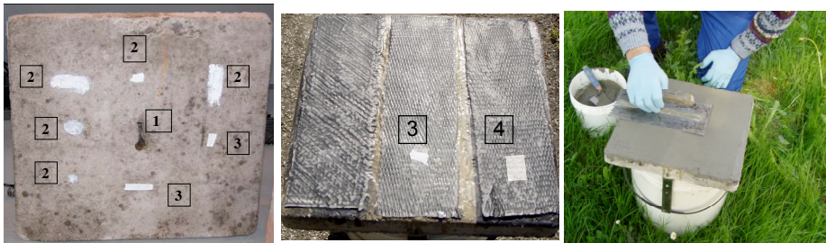
Fig. 5a. Sample setting up, concrete with different inclusions and a cavity Fig. 5b. Sample with 3 CFRP bands placed on concrete and 2 inclusions Fig. 5c. Finishing of the sample with a cement based plaster layer
