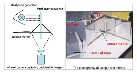
Fig. 1. Thermal measurement setup
