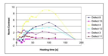
Fig. 14 Normalized contrast variation with heating time
