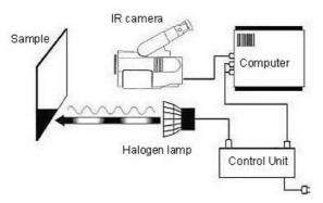
Fig. 7 Schematic illustration of LT system
