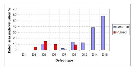
Fig. 15 Lock-in and pulsed thermography comparison
