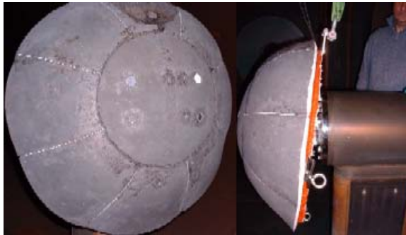
Fig. 6. NASDA Hyflex test sample. The instrumented sensors (temperature, heat flux and catalytic sensors) can be noticed on the stagnation hemispherical nose.
