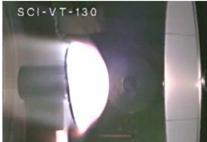
Fig. 8. NASDA Hyflex test sample under test in flow condition H1 (Table 1)
