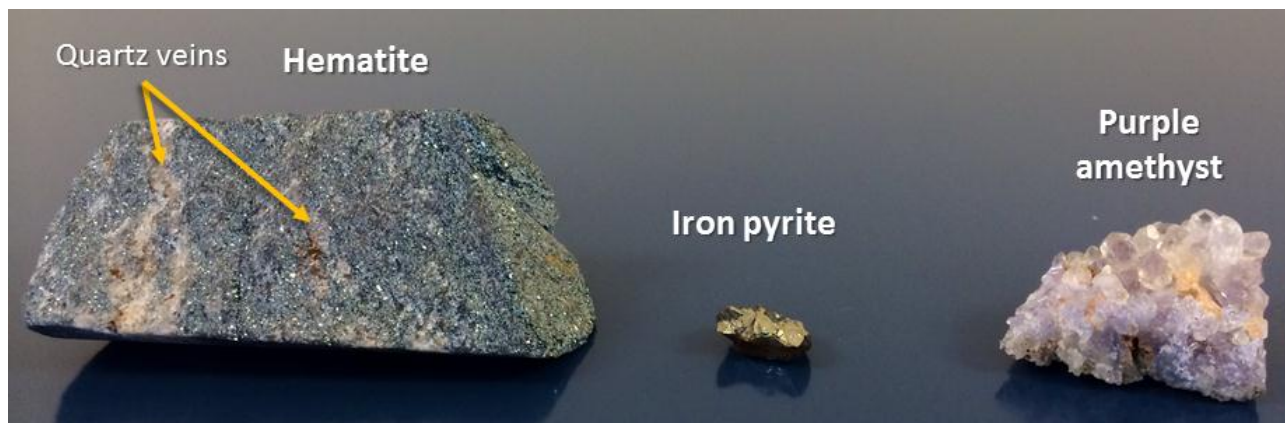
Figure 7 Visible image of a hematite drill core contaminated with quartz veins (left), iron pyrite (center) and amethyst (right).
