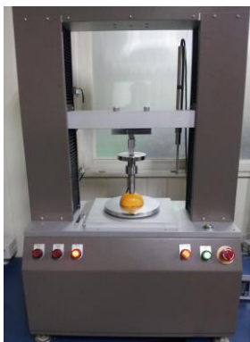
Fig. 1. Universal testing machine used in the application of force to a persimmon
