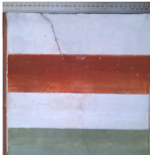
Fig. 2. Fresco specimen made with traditional techniques. The specimen width and height are equal respectively to 0.34 and 0.41 m.
