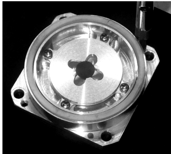
Fig. 7. A hanging microchannel silicon membrane mounted in the container (cell).
