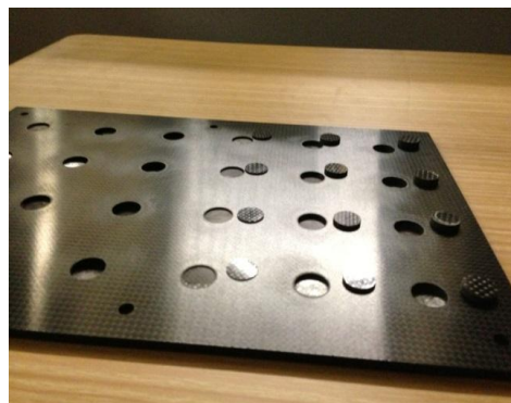
Figure 2: Inserts removed to apply adhesives
