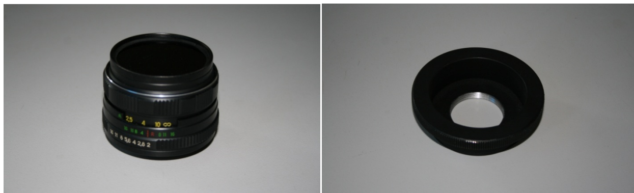
Fig. 5. Helios 44M lens with an IR filter (left) and the M42 to M80 adapter (right) used for research
