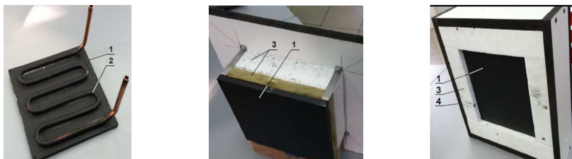
Fig. 2. Construction of main heating/cooling board; 1-copper board, 2-tortuous tube for cooling/heating agent, 3-thermal insulation, 4-external casing
