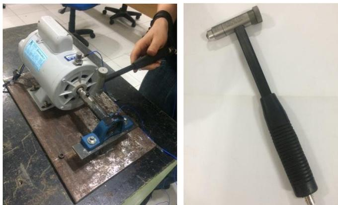
**Fig. 5.** Excitation System (left). Impulse force Hammer Test (right).
