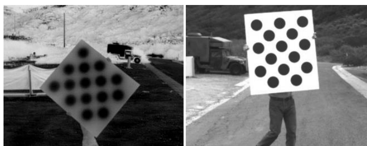
Fig. 2. Thermal (left) and visible (right) image of Dibond® asymmetric calibration rig proposed by Harguess et al. [7].
