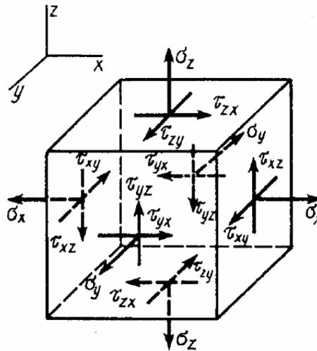
Fig. 5. Stresses acting on a test sample of elementary volume.
