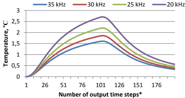
**Fig. 8.** Change in the signal temperature above the defect D1 at different frequencies for a model of sandwich plate with a polyurethane foam core (\*time step 0.05 s).
