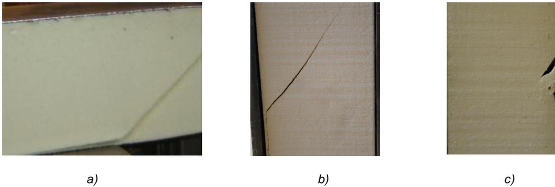
**Fig. 2.** Various types of cracks caused by: a) bending test b) and c) double lap shear test
