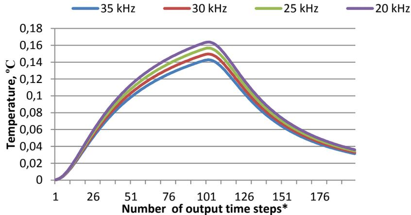
**Fig. 9.** Change in the signal temperature above the defect D1 at different frequencies for a model of sandwich plate with a mineral wool core (\*time step 0.05 s).
