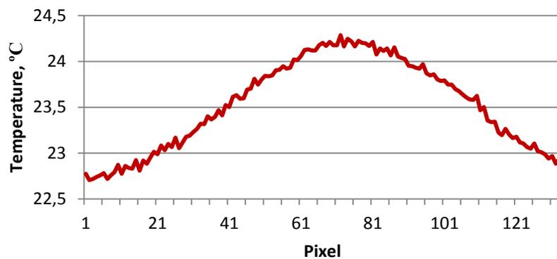
**Fig. 11.** Temperature changes on the surface of the sheet above the defect visible on the thermogram Fig. 10
