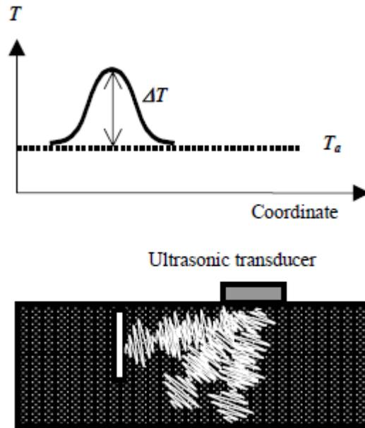
Fig. 4. Ultrasonic IR thermography principle.
