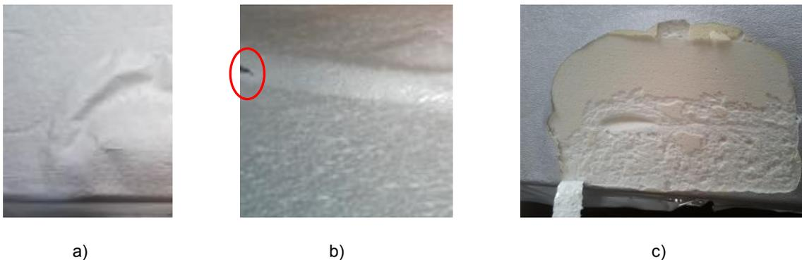
**Fig. 3.** Various types of blisters : a) blister b) blister with failure of face sheet c) the visible core after removing the blister.
