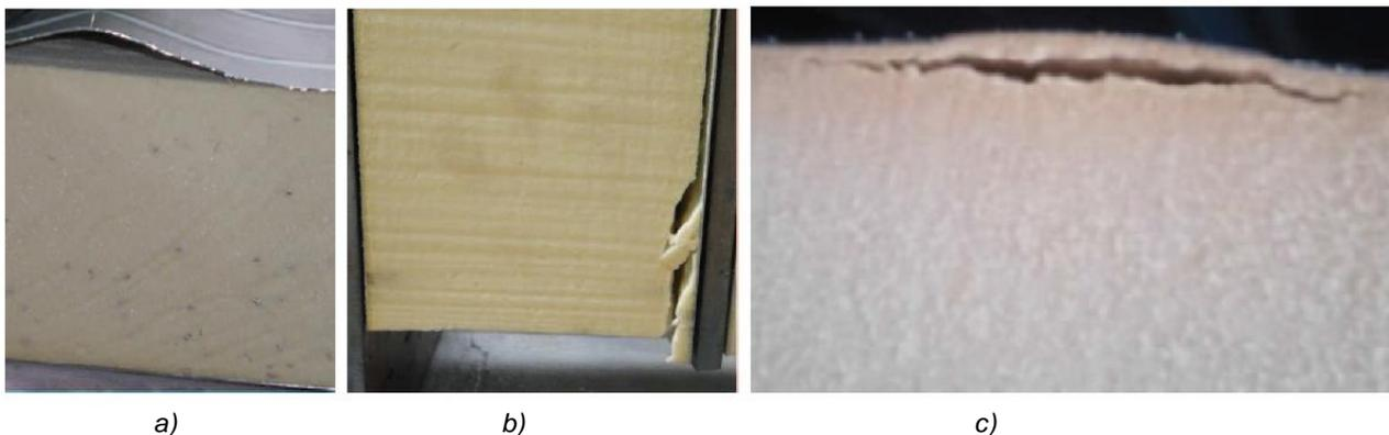
**Fig. 1.** Various types of delamination caused by: a) bending force, b) shear force, c) pressure
