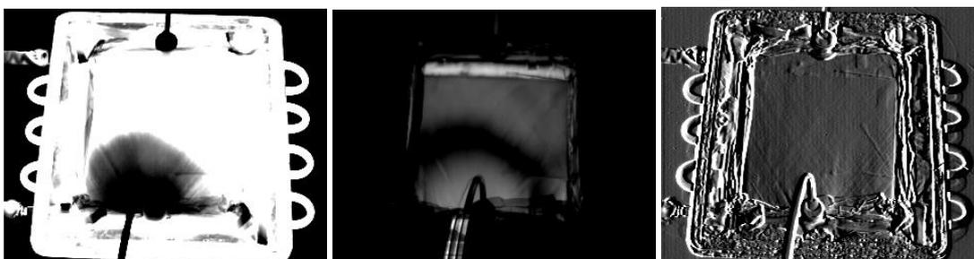
*Fig. 8. Detection of foreign material inclusions during resin injection stage. Temporary analysis of temperature (left), modulus of Fourier analysis (center) and first order gradient in x coordinate (right).*
