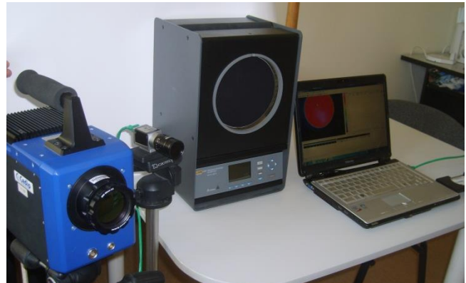
Fig. 7. Stand for the CCD-NIR camera calibration
