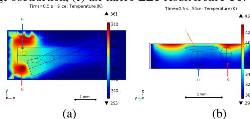
Figure 2: Slice temperature distribution when the heating time is 0.5 s: (a) top view, (b) side view.
