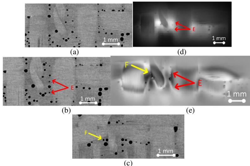
Figure 1: The comparison of micro-CT and micro-LLT results from the position of 129 mm: (a) the micro-CT slice on surface, (b) the micro-CT slice from the depth of  $36 \mu\text{m}$ , (c) the micro-CT slice from the depth of  $0.162 \text{ mm}$ , (d) the micro-LLT result from cold image subtraction, (e) the micro-LLT result from PCT.
