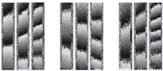
2kN3kN4kN2kN3kN4kN2kN3kN4kN(a)140A(b)160A(c)180AFig. 6 Results of the residual stress measurement using ESPI with MTS tensile testing machine.
