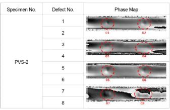
Fig. 8 Results of the inner defect detection of a pipe in heating circulation system using shearography and cooling system.
