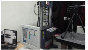
**Fig. 5** Experimental ESPI setup for measuring residual stress on the welded specimen with MTS tensile testing machine.
