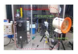
**Fig. 7** Experimental Shearography setup for detecting inner defect of a pipe in heating circulation system.
