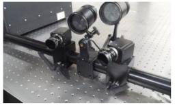
Fig. 2 Experimental DIC setup using stereo vision for measuring tensile stress on the standard tensile specimen.
