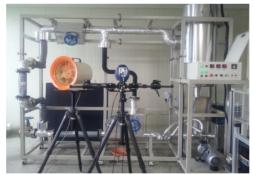
Fig. 1 Experimental IR setup for detecting inner defect of a pipe in the heating circulation system.
