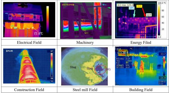
Figure 1. Equipment diagnosis case using infrared imaging camera
