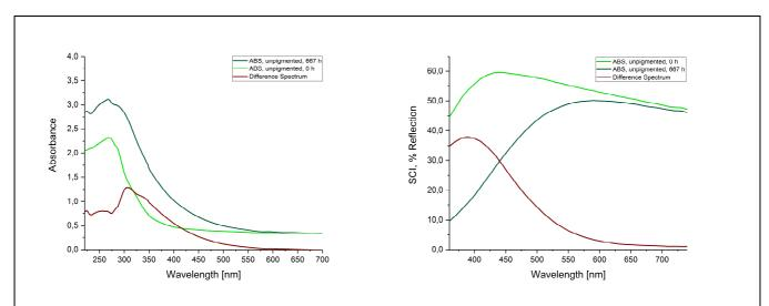
Fig. 3. UV/VIS spectra (left) and spectral reflection data (right) for a 1 mm thick step of unpigmented ABS after production with AM (light green), after 667 hours of artificial weathering (dark green) and the difference spectrum (red).
