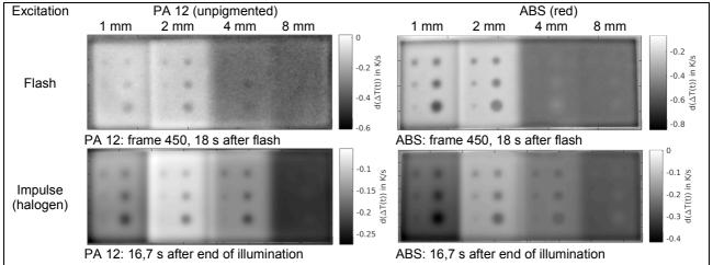
Fig. 5. Images of the first, time derivative of the thermal sequences of additively manufactured step wedges at the time of the maximum contrast of the deepest visible defects after excitation. Data processing: subtraction of zero images, appliance of a hmf and calculation of the first derivative of the thermal signal reconstruction (TSR).
