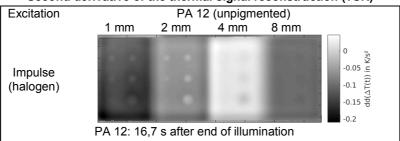
**Fig. 6.** Thermogram the PA 12 step wedge at the time of the maximum contrast of the deepest visible defects after excitation. Data processing: subtraction of zero images, appliance of hmf and calculation of the second, time derivative of the TSR.
