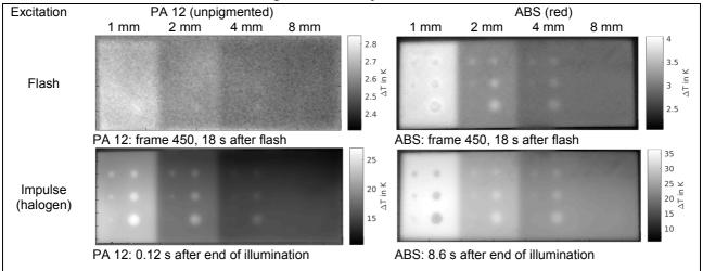
**Fig. 4.** Thermograms of additively manufactured step wedges at the time of the maximum contrast of the deepest visible defects after excitation. Data processing: subtraction of zero images, appliance of hybrid-median-filtering.
