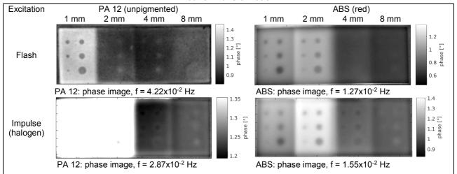
**Fig. 7.** Phase images of the thermal sequences of additively manufactured step wedges. Data processing: subtraction of zero images, appliance of hmf, thermal signal reconstruction (TSR) and Fourier-Transformation. The frequency of the maximum contrast of the deepest visible defects after excitation is shown.
