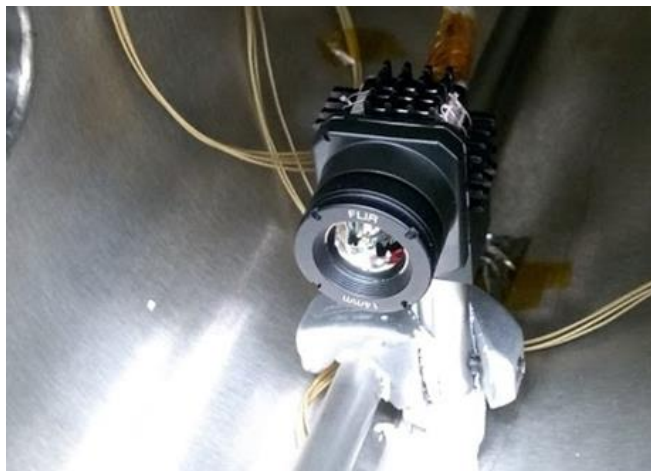
Fig. 3. Modified Boson thermal imager in place within vacuum chamber
