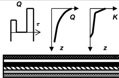
A heating function time profile  $Q(\tau)$  is defined in table form. Heating energy  $Q(z)$  is exponentially decaying with depth. Material thermal conductivity  $K(z)$  varies linearly with depth.
