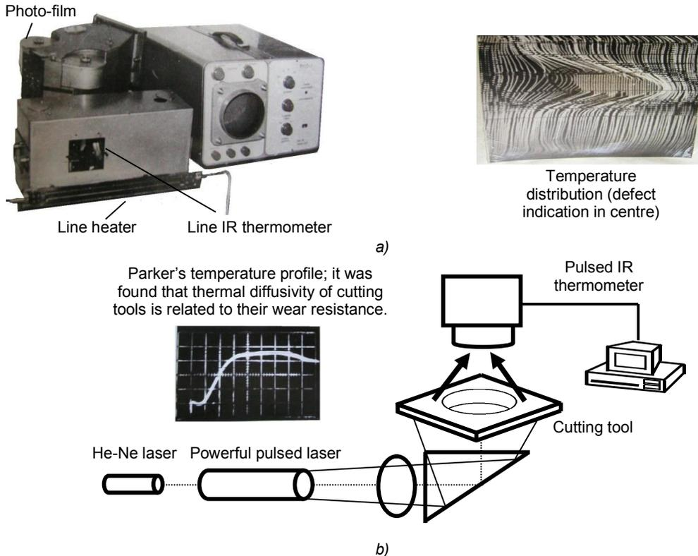
Fig. 1. Specialized TNDT equipment, Tomsk Polytechnic University:
