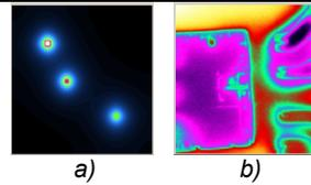
Three heat sources in a chip with no noise (a) and with imposed real-chip emissivity noise (b)
