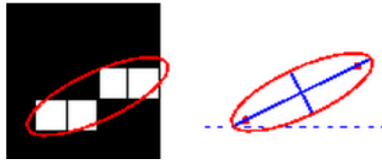
Fig. 3. Small binary image and how its orientation is calculated
