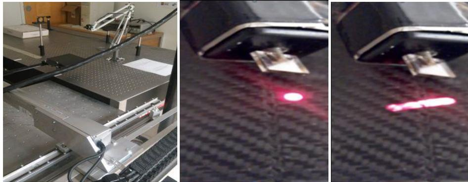
**Fig. 5.** *Micro-laser line thermography set-up*
