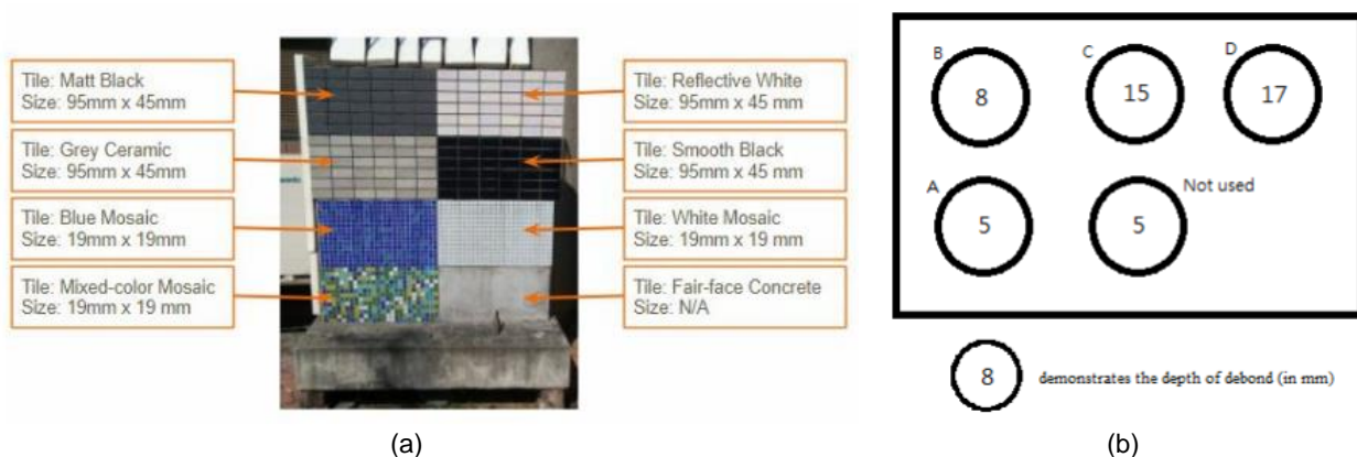
Fig. 1: (a) Details of different finishing materials on the reinforced concrete wall and (b) Demonstration of delamination with depth
