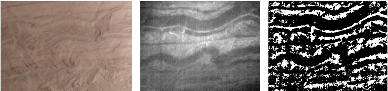
**Fig. 2:** Visual image (left); thermal image (middle) and processed image (right) of an extraction face
