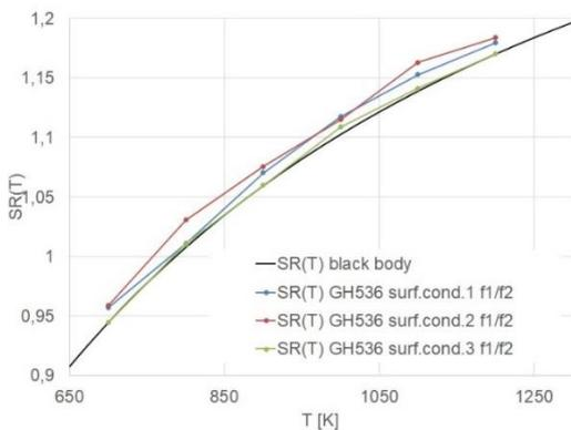
**Fig. 1:** SR curves for the couple of filters  $f_1$  and  $f_2$  without attenuator, obtained with interpolation of data coming from numerical simulation
