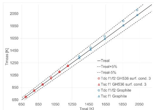
**Fig. 2:** Comparison between the two different approaches for high-emissivity materials
