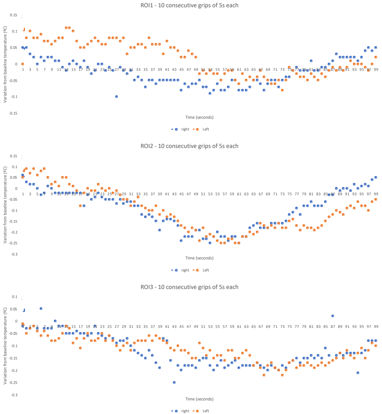
Fig. 5: The average temperature variation from baseline on the three ROIs and two forearms during the 10 consecutive grips of 5 seconds.
